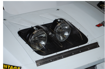
The Dzus fasteners are located near the top of the covers but beware of the header bar interference !
